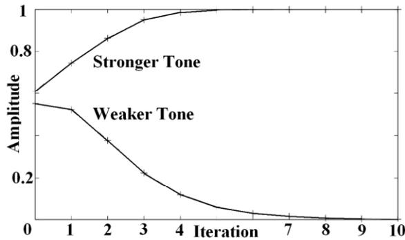
**Figure .5.**Amplitude of both complex sinusoids in the beam former output as a function of the number of LSCMA iterations. Solid line indicates predicted amplitude, '+' indicates amplitude measured in simulation.
