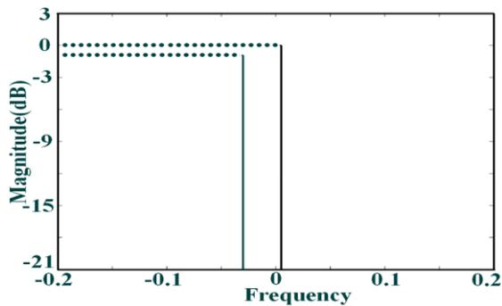
**Fig. 1.** Periodogram of the initial beam former output for the simple two-sinusoid environment. The initial SIR of 0.9 dB is indicated by the dotted horizontal lines
