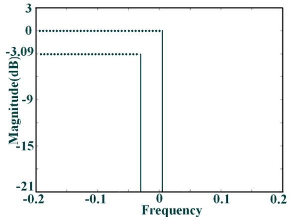
**Fig. 3.** Periodogram of the updated beam former output for the simple two-sinusoid environment. The SIR of 3.09 dB is *identical* to the SIR in the hard-limiter outputs.
