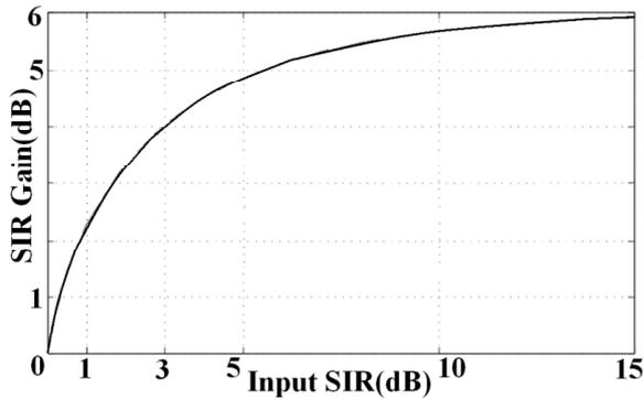
**Fig. 4.**Improvement in SIR achieved by one iteration of LSCMA with sinusoidal desired signal and sinusoidal interferer.
