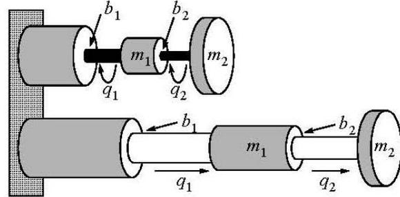
**Figure.8:** Redundant rotary & prismatic actuators.
