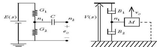
**Figure 3:** RC circuit and mechanical equivalent.
