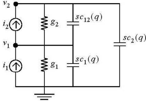
**Figure.11:** Electrical model of 2-DOF serial robot.
