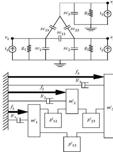
Figure.15: Model of a 3-DOF parallel robot.
