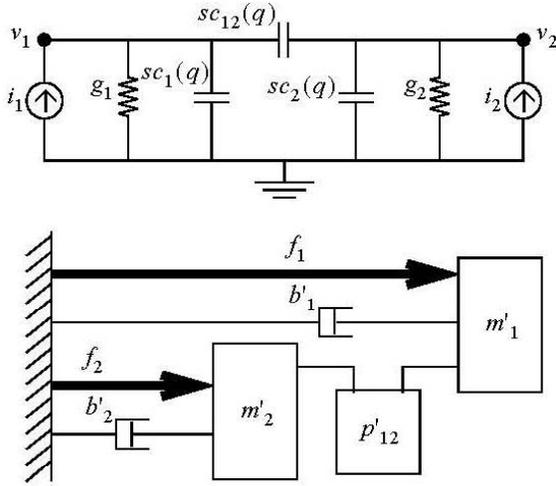
**Figure.13:** Model of a 2-DOF parallel robot.
