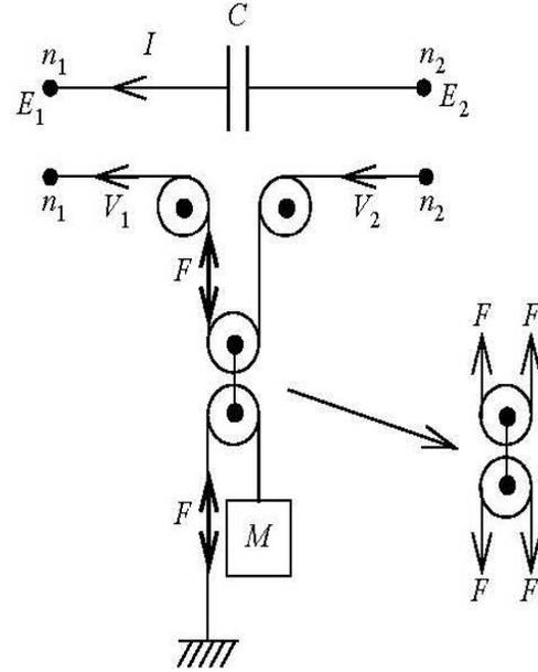
Figure. 5: Mass / pulley equivalent of a capacitor
