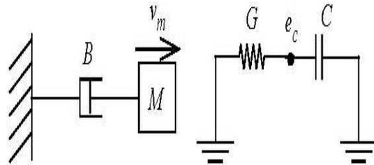
**Figure. 2:** LC circuit and mechanical equivalent.
