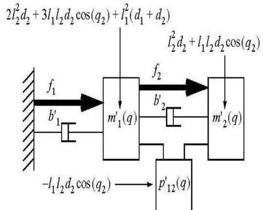
**Figure.12:** Mechanical model of a 2-DOF serial robot.
