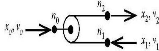
Figure. 4: Pulley based differential transmission.
