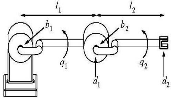
**Figure.10:** 2-DOF serial robot.
