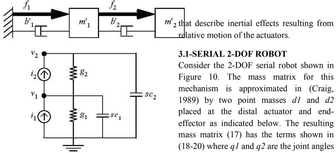
**Figure.9:** System models of redundant actuators
