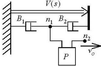
**Figure.7:** Mechanical equivalent using MP model
