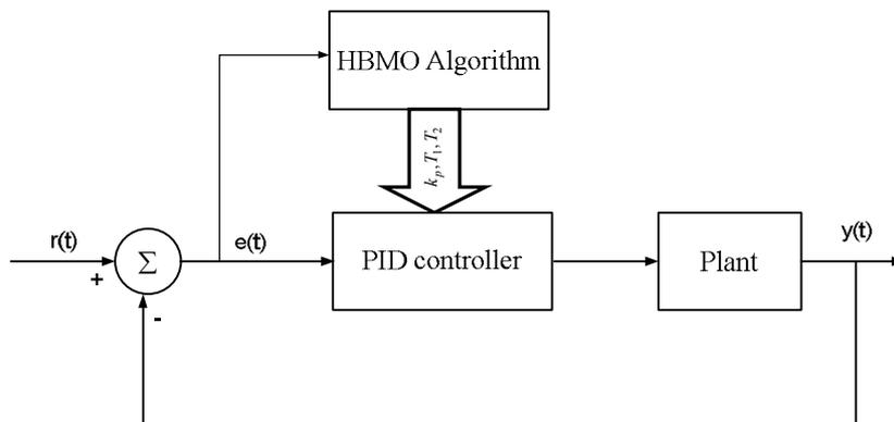
Fig. 3. Schematic of the proposed controller designing
