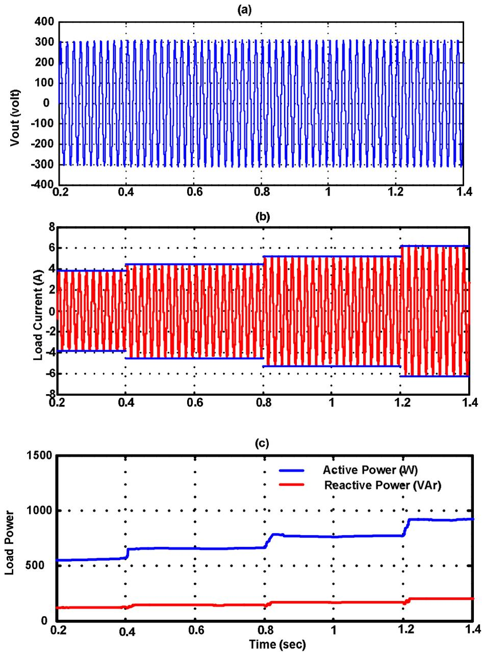
Fig. 6. System response using a conventional PID controller
