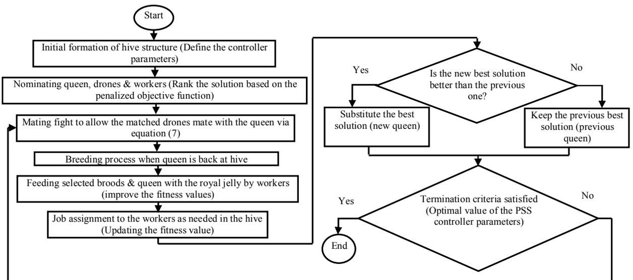
Fig. 2. Algorithm and computational flowchart of HBMO
