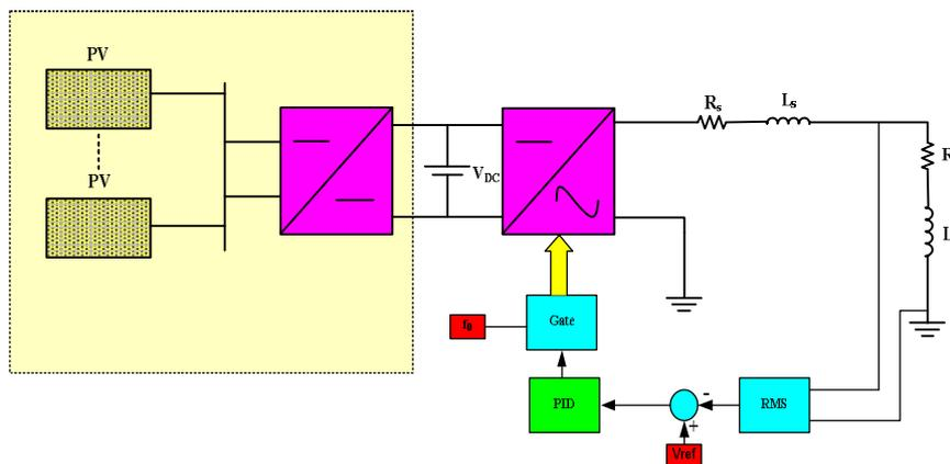
**Fig.1.** Photovoltaic system with battery, inverter and load
