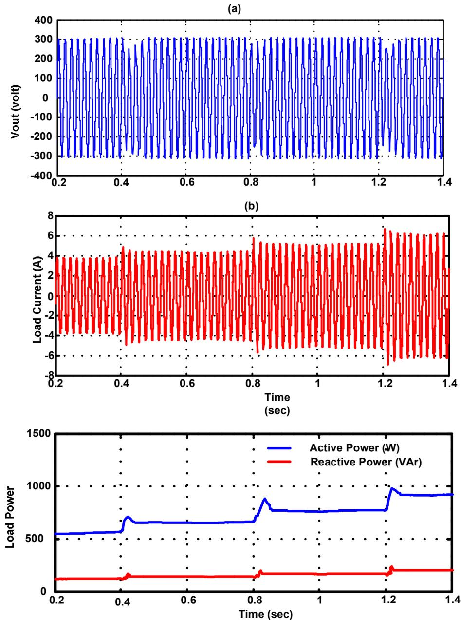
Fig.5. System response using a conventional PID controller
