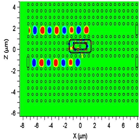
**Fig.5.** Electromagnetic field intensity for a wavelength of 1550 nm
