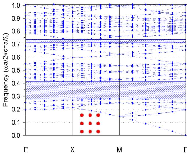
Fig.1. Band structure of the photonic crystal
