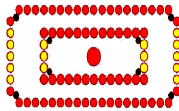
Fig.2. Display of structure of nested rectangular photonic crystal resonator
