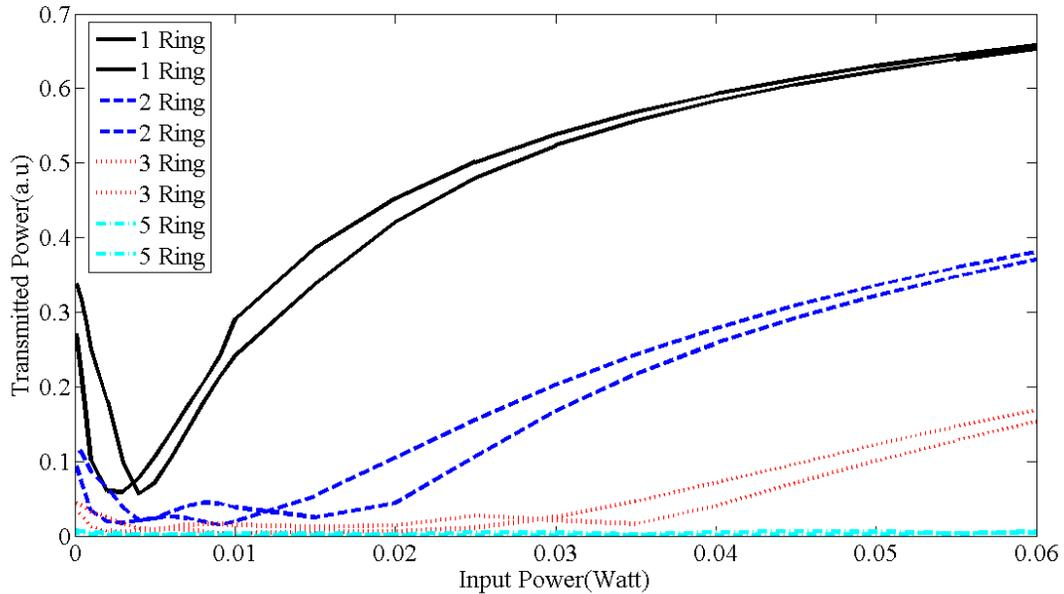
**Fig.10.** Resonator Transfer Curves for different number of rings in critical coupling Condition ( $\lambda_{in}=1550\text{nm}$ )
