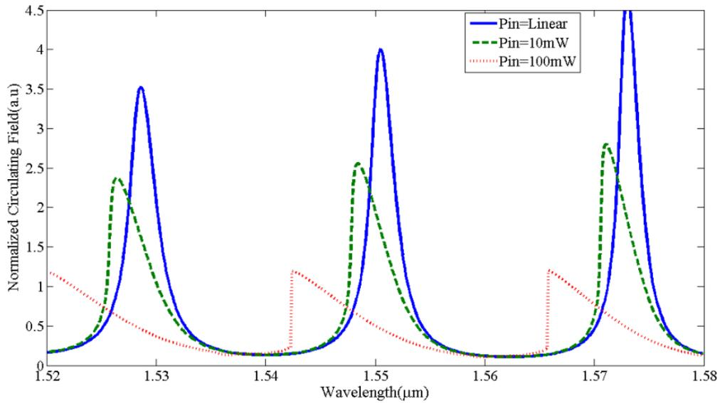
**Fig.4.** Circulating Spectral Response of a single-ring Resonator for Different input power (normalized to input power)
