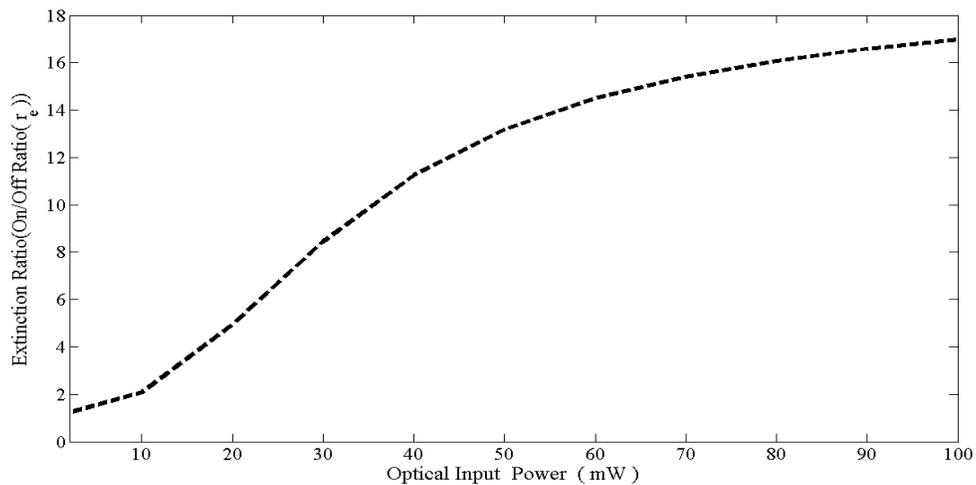
**Fig.12.** Two level Resolution vs. Different Input Optical Power
