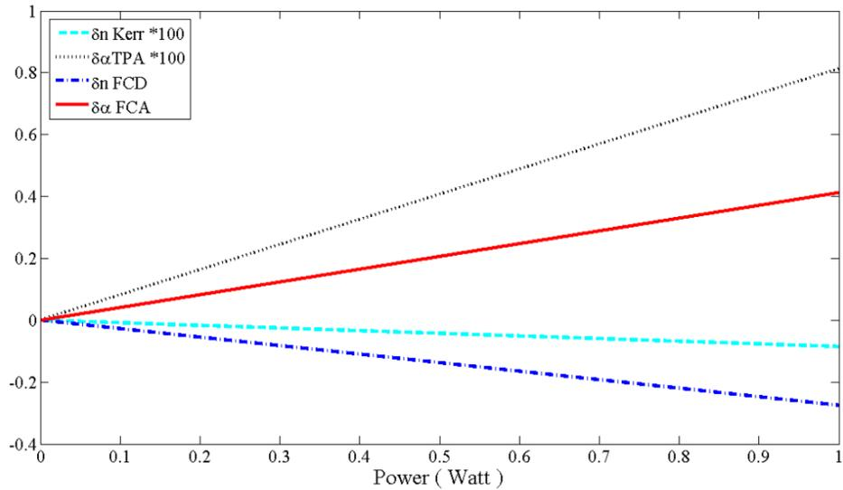
**Fig.7.** Change of refractive index and absorption coefficient for different optical power for considering any of nonlinear effects
