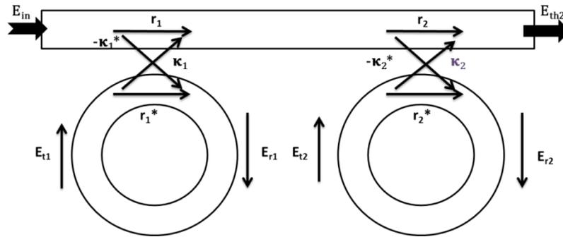
Fig.1. Double Ring-Resonator Array Simulation Model
