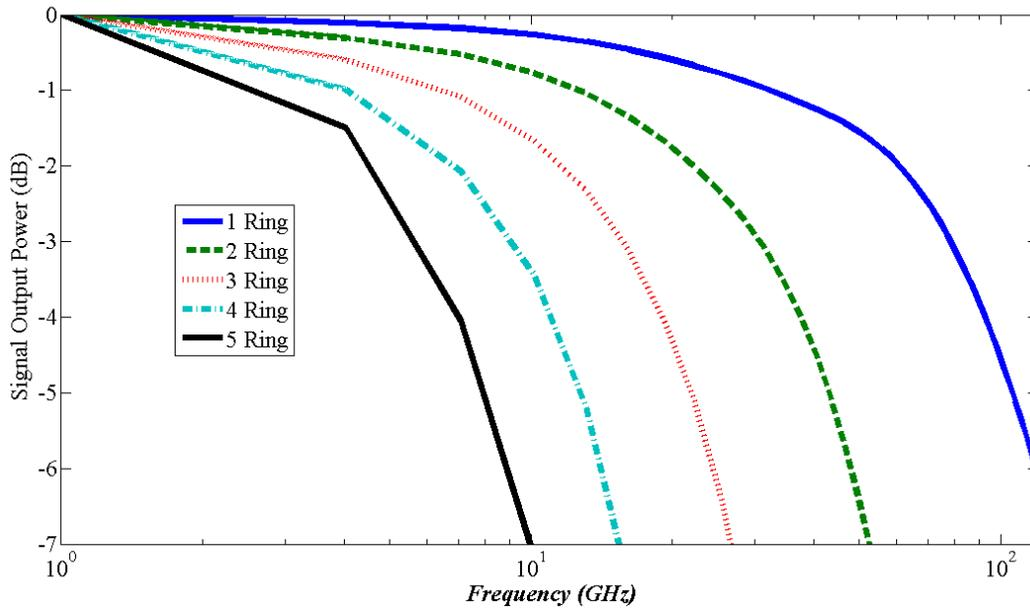
**Fig.11.** Frequency Response of Ring Resonator Array in Critical Coupling Condition for Different Number of Rings ( $\lambda_{in}=1550.9\text{nm}$ )
