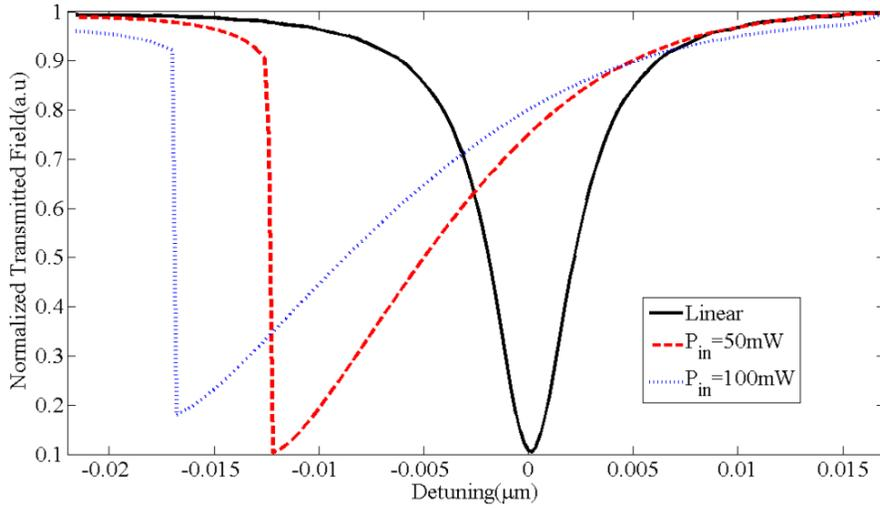
**Fig.5.** Output Spectral Response of a single-ring Resonator for Different input power (normalized to input power)
