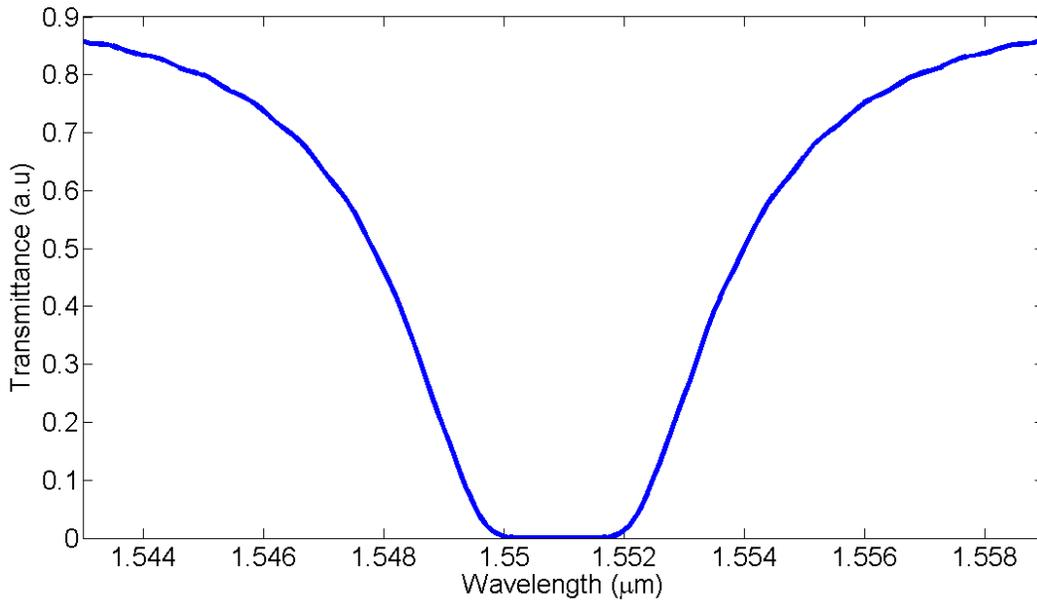
**Fig.9.** Spectral Response of 10 Ring Parallel Array in Critical Coupling Condition ( $R=5\mu$ )
