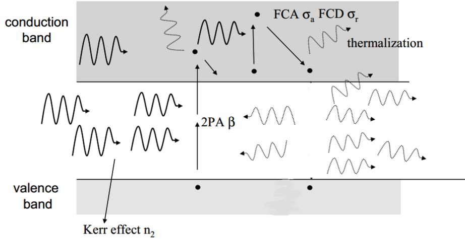
**Fig.2.** Optical Kerr, FCD, FCA and TPA effects in the InGaAs semiconductor [8]
