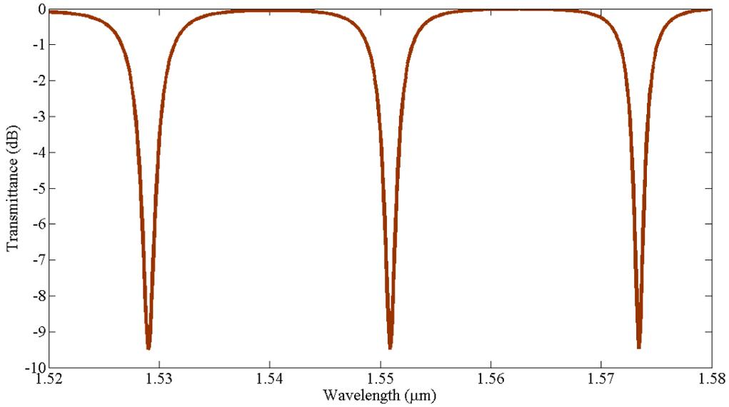
**Fig. 3.** Output Spectral Response of a single-ring Resonator ( $R=5\mu\text{m}$ )
