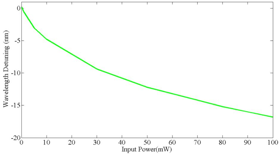
**Fig.6.** Resonance Wavelength Blue shift as a function of the input optical power
