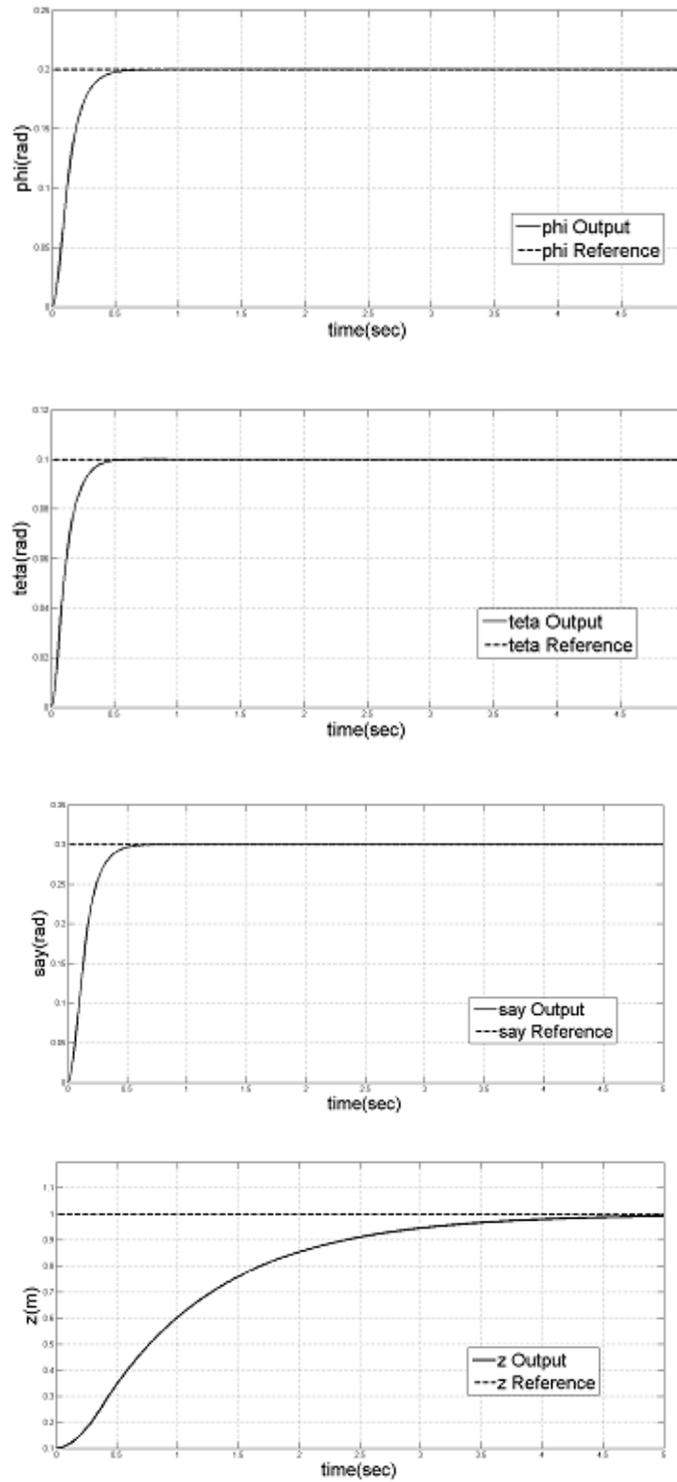
Fig. 3. The roll, pitch and yaw angles and Altitude to Arbitrary values.
