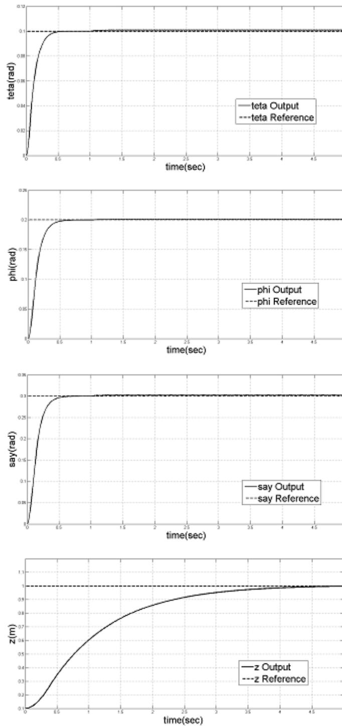
**Fig. 4.** The roll, pitch and yaw angles and Altitude to Arbitrary values.
