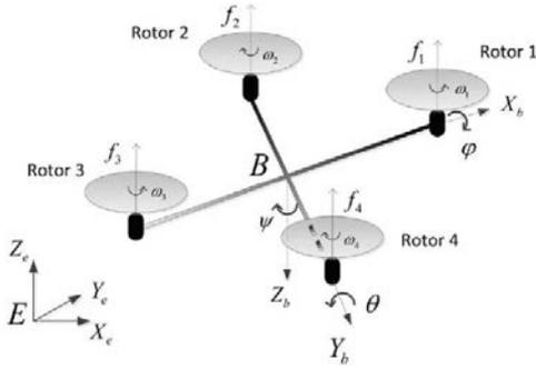
**Fig.1.**Schematic view of quadrotor aircraft
