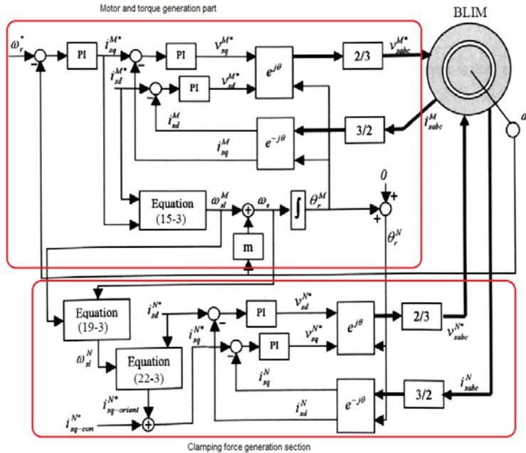
Fig. 1. Overall scheme of the vector control of the BLIM
