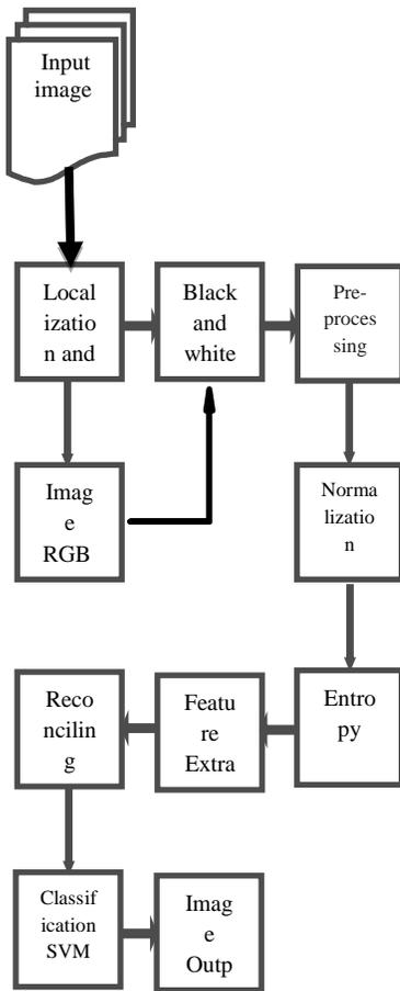
**Fig .2.**Block diagram of the proposed face recognition system in this paper
