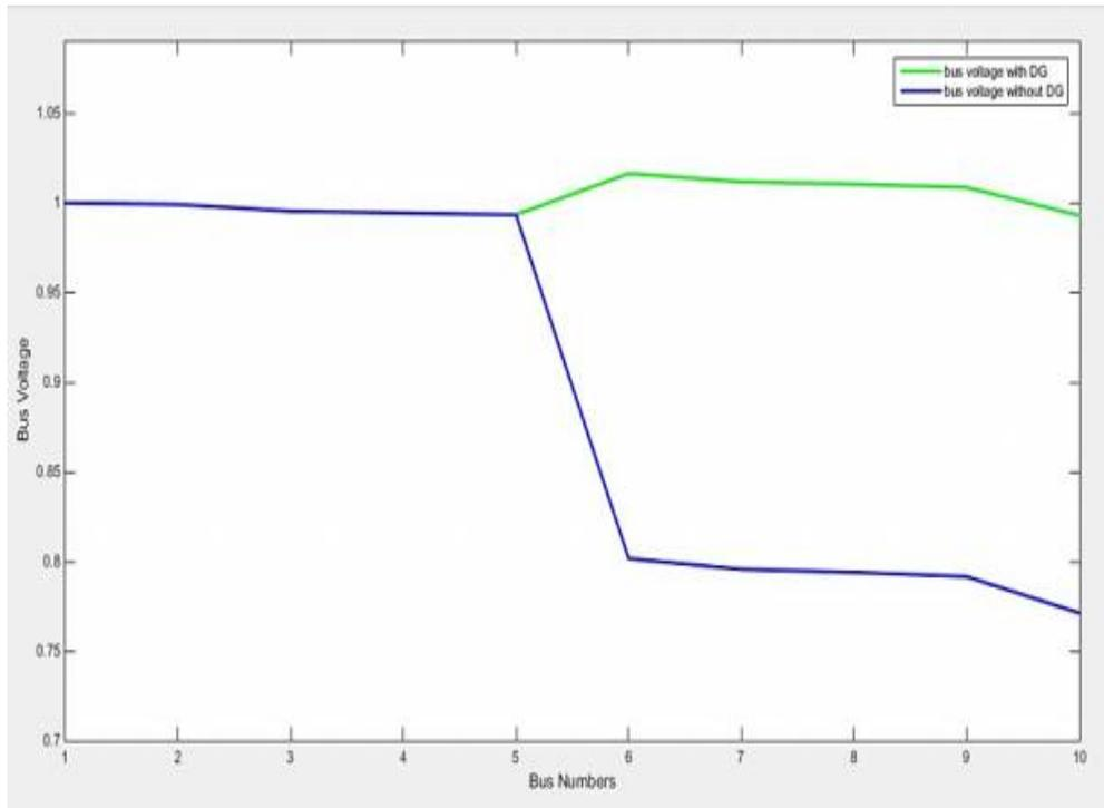
Fig .3. Voltage profile comparison before and after DG installation in 10-bus network
