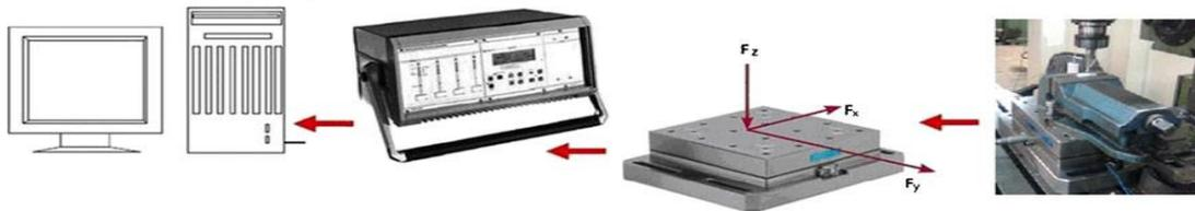
Fig.1.schematic layout of axial force measurement
