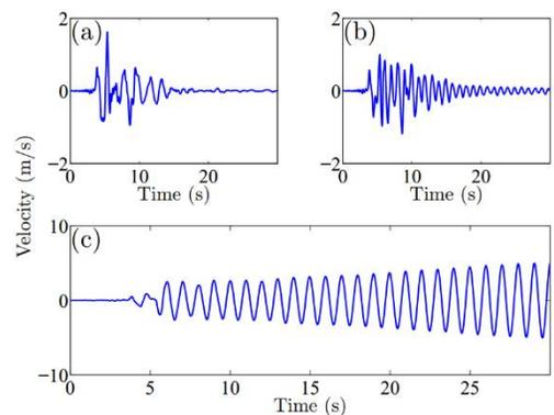
**Fig.6.** Velocity of the structure subjected to Newhall; (a) controlled with SMC, (b) controlled with ASMC, (c) uncontrolled.
