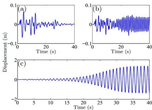
**Fig.3.** Displacement of the structure subjected to El-Centro; (a) controlled with SMC, (b) controlled with ASMC, (c) uncontrolled.
