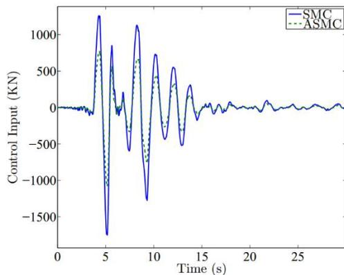
**Fig.8.** Control Force (KN), when the structure is subjected to Newhall earthquake.
