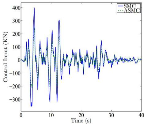
**Fig.7.** Control Force (KN), when the structure is subjected to El-Centro earthquake.
