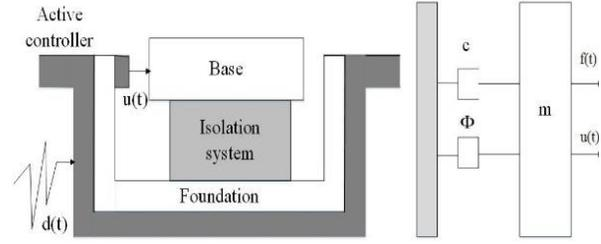
**Fig.1.** Base isolation system (left) and schematic model (right)
