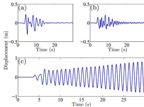
**Fig.5.** Displacement of the structure subjected to Newhall; (a) controlled with SMC, (b) controlled with ASMC, (c) uncontrolled.
