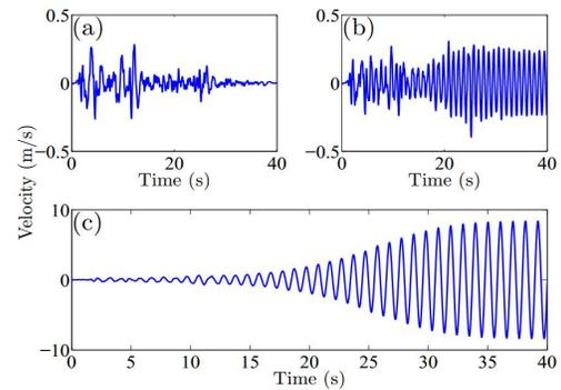
**Fig.4.** Velocity of the structure subjected to El-Centro; (a) controlled with SMC, (b) controlled with ASMC, (c) uncontrolled.
