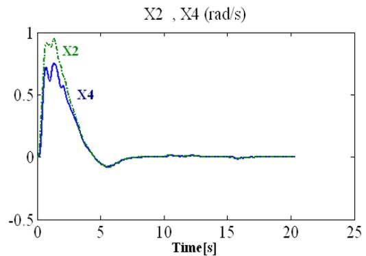
**Fig.3.** Arm speed ( $x_2$ ) and driver ( $x_4$ ) in a number of experiments
