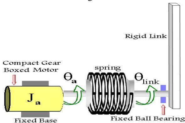
**Fig.1.** Single-armed FJR schematic
