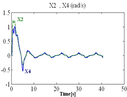
**Fig.5.** Arm speed ( $x_2$ ) and driver ( $x_4$ ) in test 2
