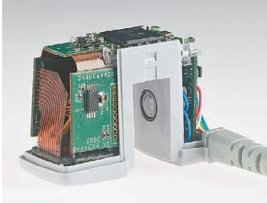
Fig.10. The Internal Circuitry Capnograph Sensor (sensor CO_2 )
