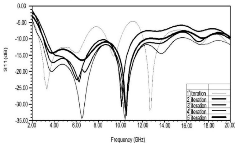
**Fig.3.**The simulated curves for five iterations of fractal
