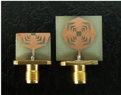
**Fig.10.** Photograph of the comparison between both fabricated antennas
