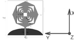
**Fig.1.** Geometry of a fifth iteration of fractal micro-strip antenna for UWB uses.
