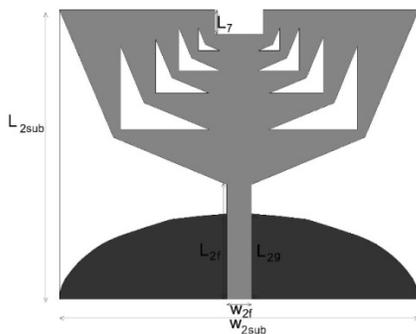
**Fig.6.** Geometry of the proposed miniaturized antenna
