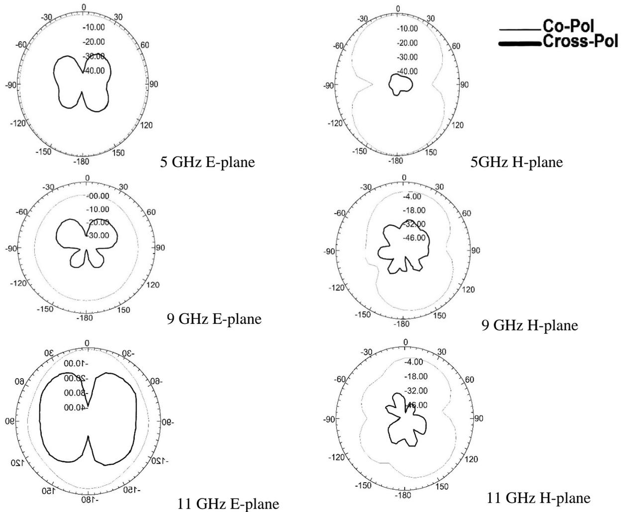
**Fig.4.** Measured E-plane and H-plane radiation patterns of proposed antenna at 5, 9, and 11 GHz
