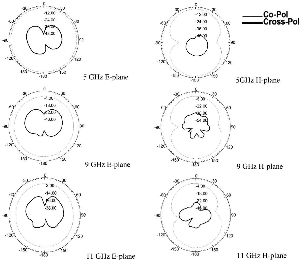
**Fig.9.** Measured E-plane and H-plane radiation patterns of miniaturized antenna at 5, 9, and 11 GHz
