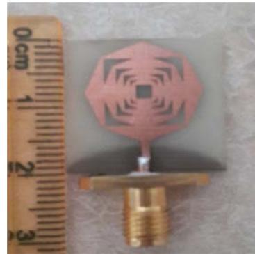
**Fig.2.** Photograph of the fabricated Fractal patch Antenna
