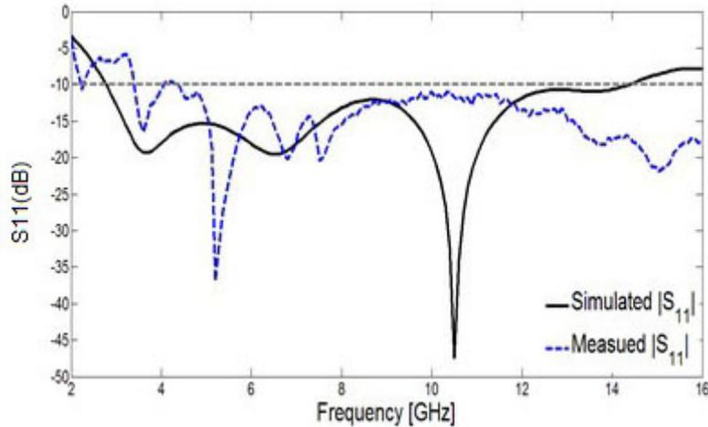
**Fig.5.** Simulated and measured S11 for five iteration of fractal
