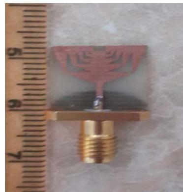
**Fig.8.** Photograph of the fabricated miniaturized antenna
