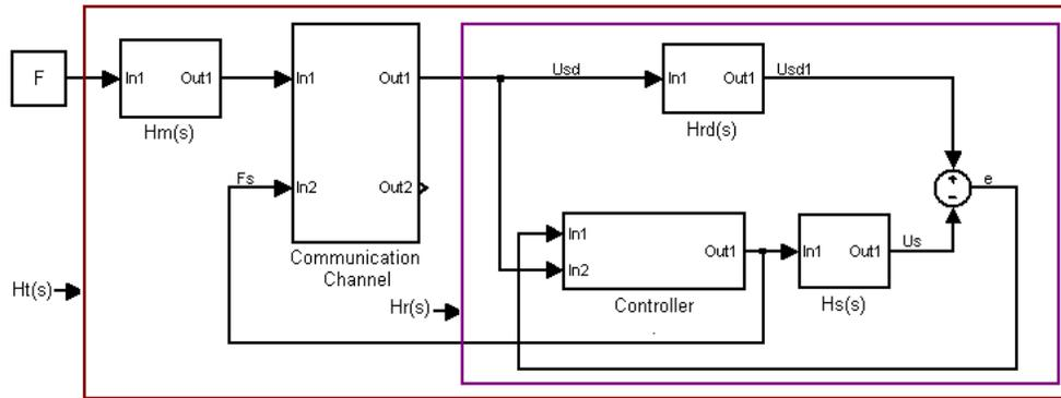
**Fig.1.** The model reference adaptive controller
