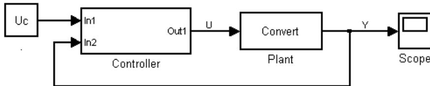
Fig.2. block diagram PID controller
