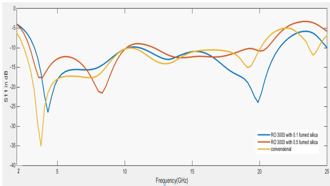
**Fig.4.** S<sub>11</sub> plot of conventional antenna and antenna with substrate of RO3003 with 0.1 and 0.5 fumed silica
