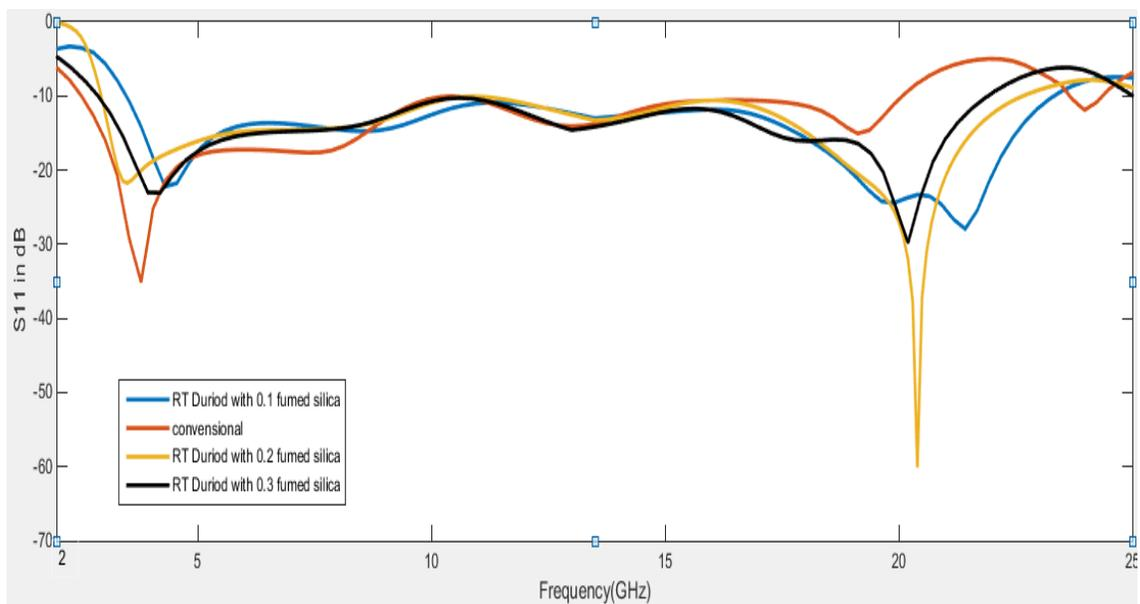
**Fig.2.** S<sub>11</sub> plot of conventional antenna and antenna with substrates of RT Duriod 5880 with 0.1 Fumed Silica, 0.2 Fumed Silica and 0.3 Fumed Silica
