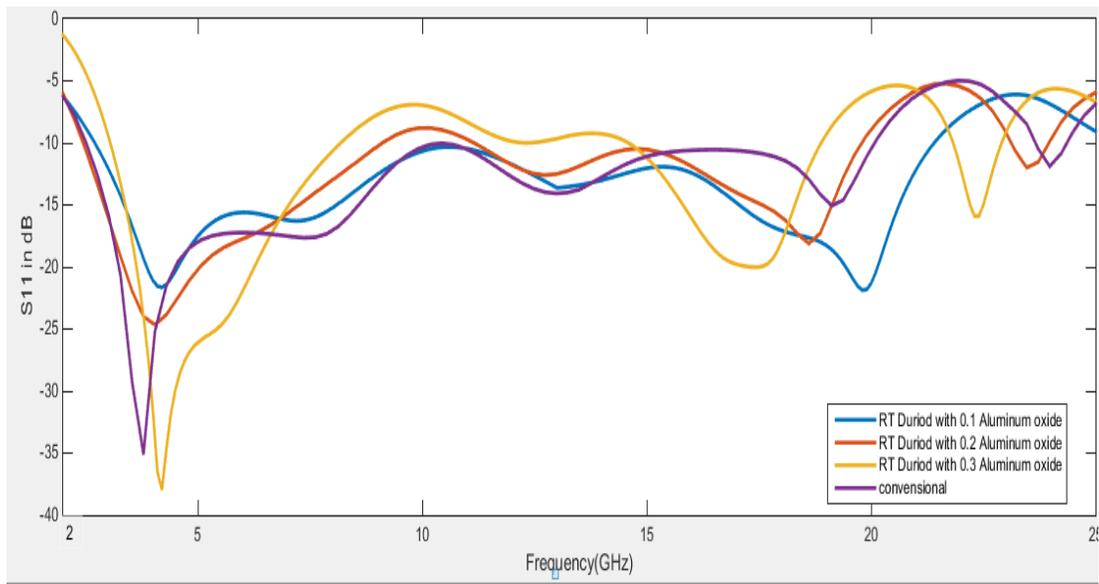
**Fig.3.** S<sub>11</sub> plot of conventional antenna and antenna with substrates of RT Duriod 5880 with 0.1 Aluminum Oxide, 0.2 Aluminum Oxide and 0.3 Aluminum Oxide
