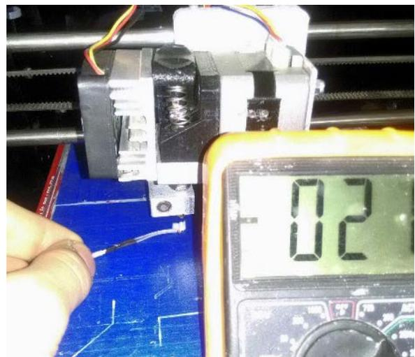
**Fig. 2.** Object resistance after temperature equilibrium
