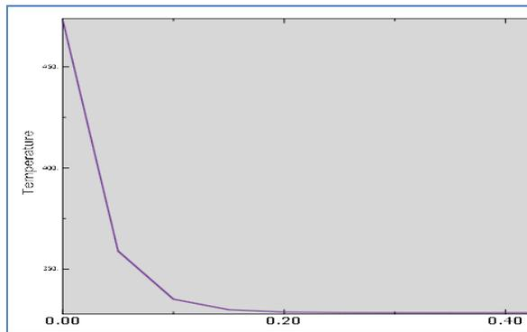
**Fig. 10.** The graph of temperature changes based on time for central node of lower plate
