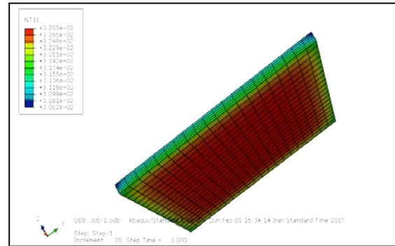
**Fig. 7.** Temperature contour after one second (under the object)
