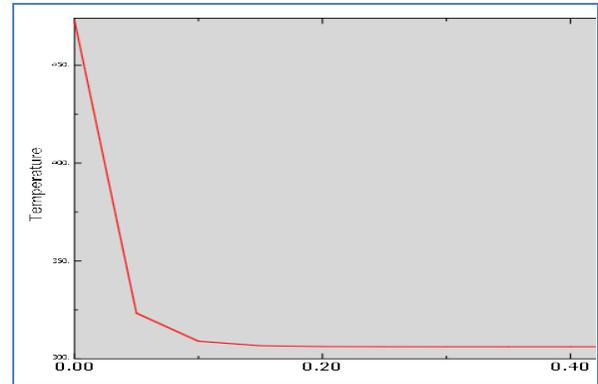
**Fig. 8.** The graph of temperature changes based on time for corner node of upper plate
