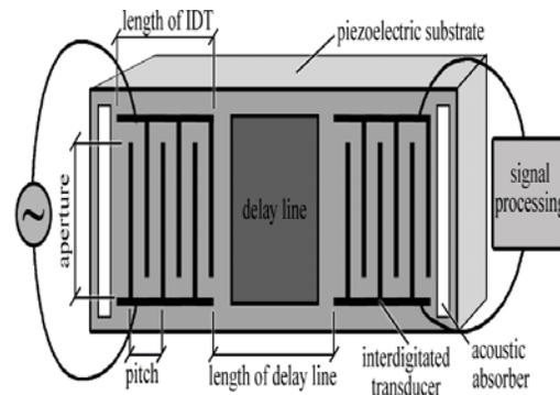
**Fig.1.** SAW waveguide
