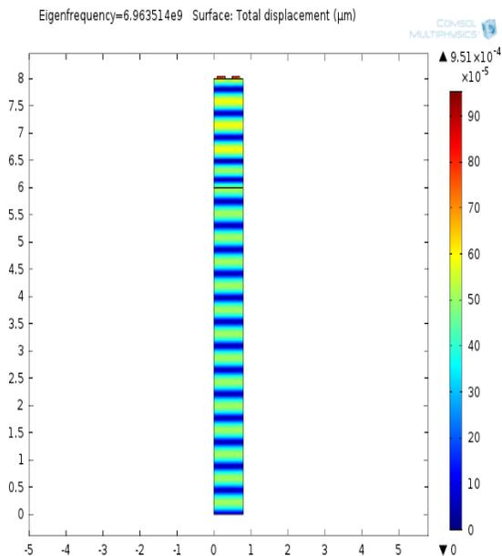
**Fig.4.** The structure response at a frequency of 6.96 GHz and viewing volumetric waves
