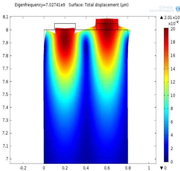
**Fig.3.** Mode aluminum nitride and gallium nitride anti-resonance in the substrate mix
