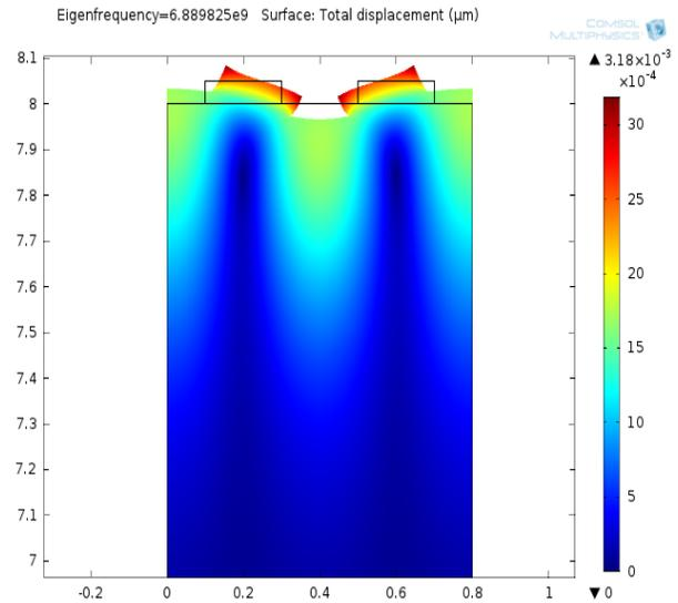
**Fig.2.** Resonant mode in the substrate of aluminum nitride and gallium nitride
