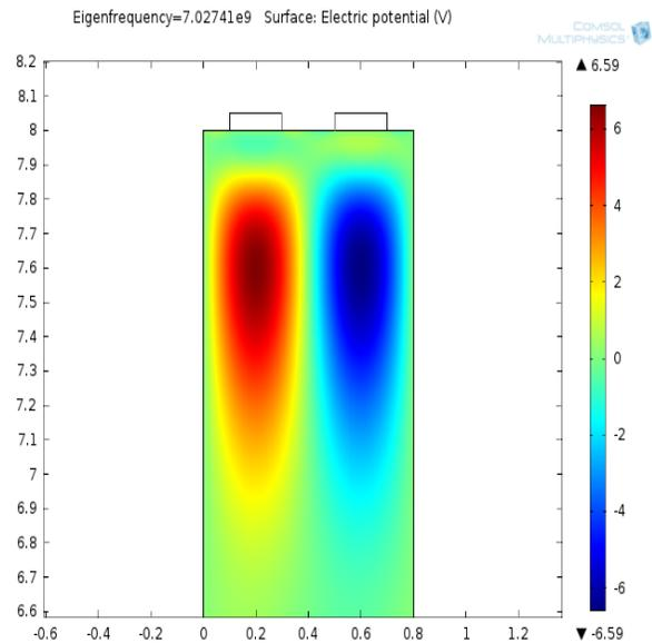
**Fig.5.** The electric potential at a frequency 7.027 GHz
