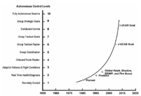
**Fig.1.** The control independence level and aircraft independence trend
