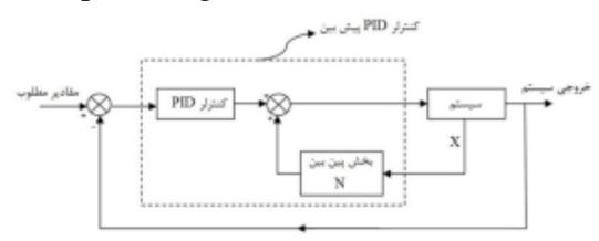
Fig.4. Block diagram of predictive PID controller
